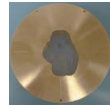
Beams may be aimed from multiple directions to treat a lesion. A Brass aperture is custom milled and shaped to the profile of the lesion for each beam used. The Brass stops the protons ensuring that only the intended lesion is irradiated minimizing the dose received by nearby normal tissue.
